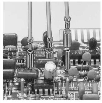
This terminal is used with 2.36mm (.093") diameter GT pins. The SPF terminal has a large contact area, withstands stress caused by repeated insertions and removals, and provides excellent retaining force. It is best suited for circuit connections that require a large current.
